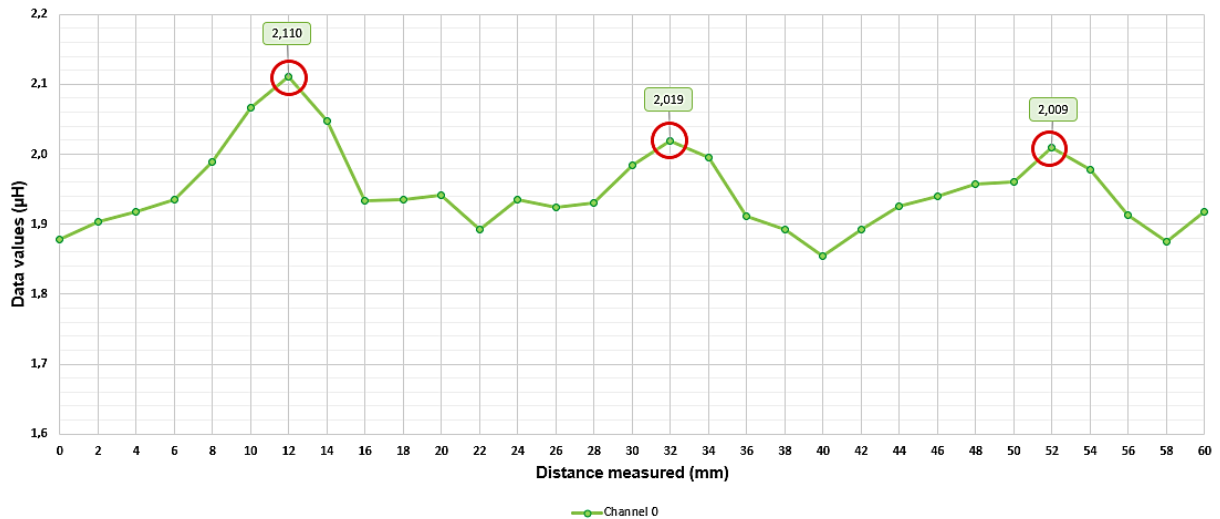
Figure 5.3 - Measurements over distance through Channel 0, perpendicular cracks.
